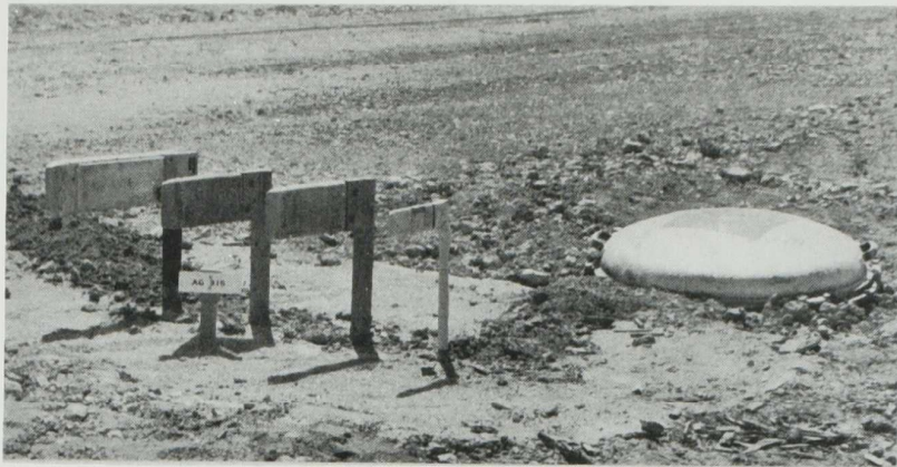
FIG. 1. BLAST GAUGE SITE , SHOWING (RIGHT TO LEFT) F.M.T. CONTAINER , F.M.T. GAUGE , TWO BAFFLES , & DIAPHRAGM GAUGE.
